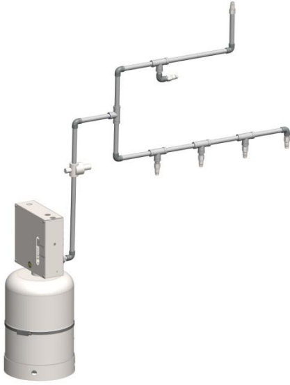
Figure 37: System example having two discharge lines
