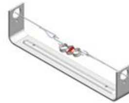
Figure 22: Thermobulb link-leg installation
