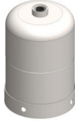
P2250 / DM12 Cylinder Capacity 15 LT Dimension 265 mm x 564 mm Material : EN 10111 DD11 Muff connection: 2" BSPP Siphon connection: 3 ¼" BSPP Operating pressure:9 bar Test pressure: 25 Bar Operating temperature: +5C / +49 C
