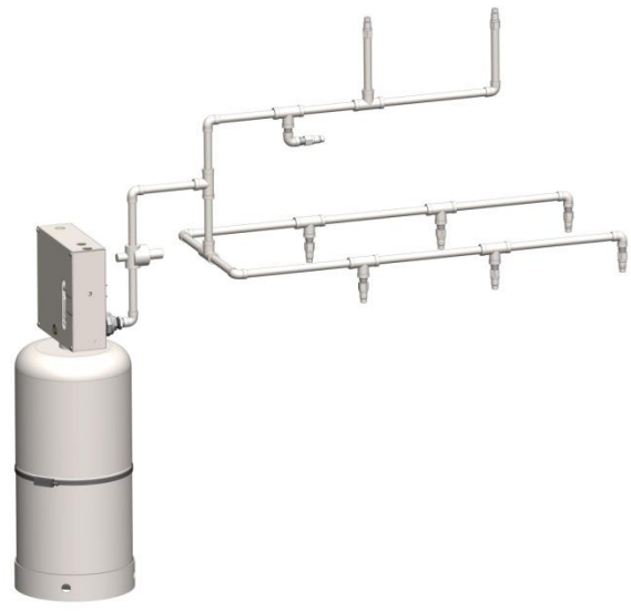
Figure 38: System example having triple discharge lines
